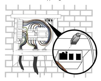
b. Mount the front plate into position by connecting the 12-pin plug to the PCB attached to the front plate. Make sure to hear a click when connecting the 12-pin plug.
