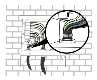
c. Mount the separate cable holder on the wall nearby the EV Wall Business. As the cable socket is situated on the righthand side of the EV Wall Business, we advise to mount the cable holder on the same side.
