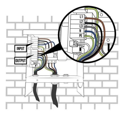
b. Mount the cable tie for strain relief on the charging cable after it enters the M32 cable gland.
