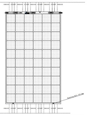
According to the actual measurement situation on the site, open the mounting hole with diameter of 5.5mm on the two short sides of the module in advance. The distance between the center of the installation holes and the edge of the component is 8-10 mm. The number of installation holes: two on each side, four in total.
