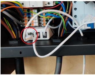
b. Mount the front plate into position by connecting the RJ10 cable to one of the B ports of the PCB attached to the front plate.
