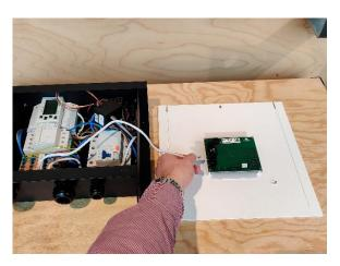
b. Attach the EV Wall Business housing to the mounting plate using the three supplied M4 x 6 mm  $\,$  HEX screws.
