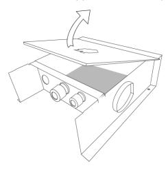
b. Attach the EV Wall Lite housing to the mounting plate using the three supplied M4 x 6 mm HEX screws.
