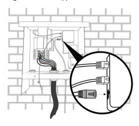
b. Mount the front plate into position by connecting the RJ10 cable to one of the B ports of the PCB attached to the front plate.
